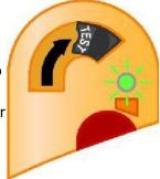
Activate Test Mode by rotating the grey test switch clockwise and holding for 1 second, until the LED indicator begins to rapidly flash Green, then release the test switch. This will initiate a self test - be prepared to monitor the number of LED indicator flashes upon completion of the test.
